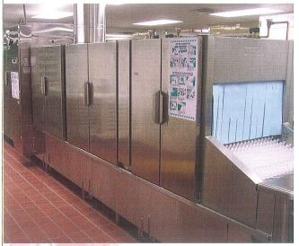
The new flight-type ware-washer features side-opening doors and easy-to-access service panels below. It's simple to service and keep clean. All the machine steam is captured through one vent and two blowers ensure wares are dry.
