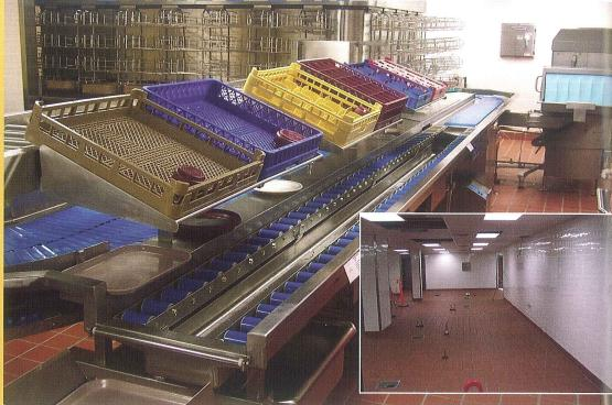
When racks are full, employees just push them onto an upper conveyor, Replacement racks are located right behind the scrappers in neat, color-coded stacks. Trays automatically feed onto a lowerater that's wheeled a couple of feet to the warewasher. Note the pulper at the end of the scrap trough
